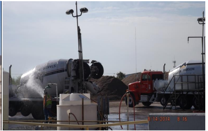
Washing down at Slump Rack
